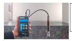
In Situ testing measures the conditions of the concrete slab at a depth of 40% of the overall thickness and gives invaluable evidence needed to ensure a good install and long lasting performance of the flooring material.
