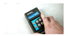
Initial non-destructive testing is vital to save time and money by mapping out the concrete slab to determine where to conduct In Situ testing under ASTMF 2170.
