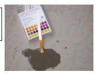
• Concrete Surface Porosity Test shall be conducted prior to the application of adhesive to evaluate bonding capacity.
